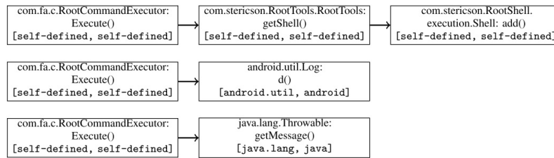
Fig. 4: Sequence of API calls extracted from the call graphs in Fig. 3, with the corresponding package/family abstraction in square brackets.
